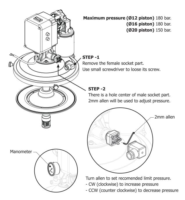
Adjusted pressure value can be controlled by manometer on pump outlet.
