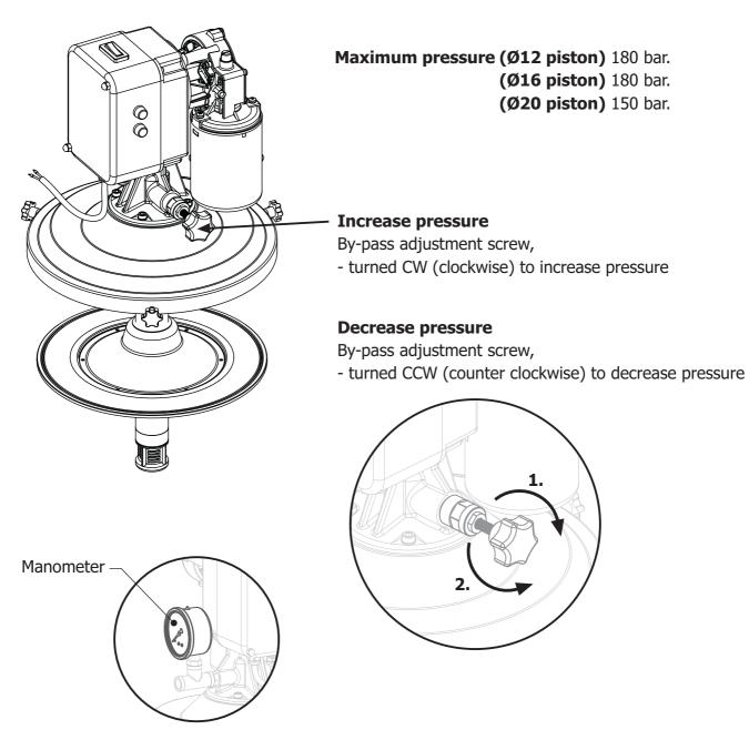
Adjusted pressure value can be controlled by manometer on pump outlet.
