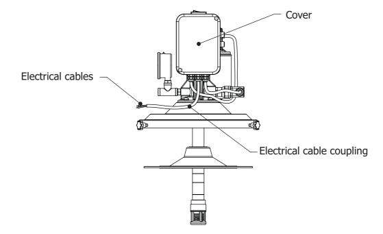
**3.** Electrical cables are marked with (+) and (-) signs. 24 V DC electrical energy should be connected as it.
