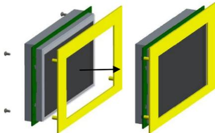
The touch TP is physically pasted on the sheet metal shell. In the cabinet design, the TP should not be suspended to prevent falling off. It is suggested that a buffer foam with a width of less than 5mm can be added at the front edge of touch TP (too large to block the LCD effective display area) to pad between the cabinet and the touch TP to form appropriate extrusion, so as to achieve the auxiliary reinforcement effect of touch TP.
