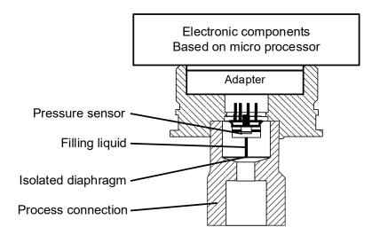
Pressure transmitter includes two functional units:
