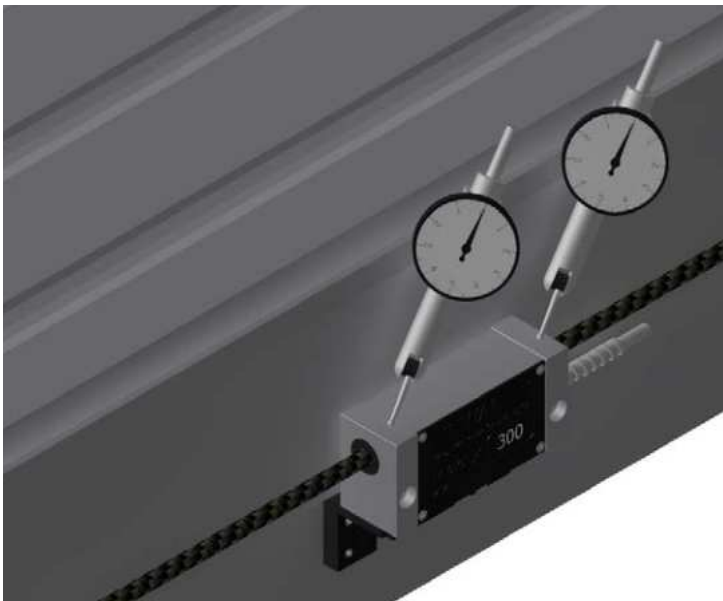
Figure 4.2 - Alignment of the Microsyn 300 Reader Head
